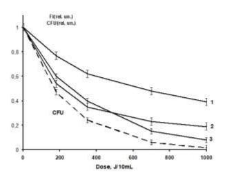
Dependence the fluorescence of tyrosine (1), albumin (2) and tryptophan (3) on the irradiation dose by the IR10 generator one day after treatment. Fl (rel. un.) – fluorescence, relative units; The fluorescence of the initial untreated solutions is taken as a unit. CFU is the relative number of colony-forming units for the bacterium *Aspergillus Niger* after treatment by the IR10 generator, the CFU value in the initial untreated solution is taken as a unit.
