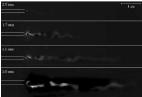
Figure 1. A composition of video frames of microwave discharge at different pressures in the flow. Frame exposure is 2 \mu\text{s} . The air flow velocity is 200 m/s, directed from left to right. The field strength vector E is parallel to the flow.
