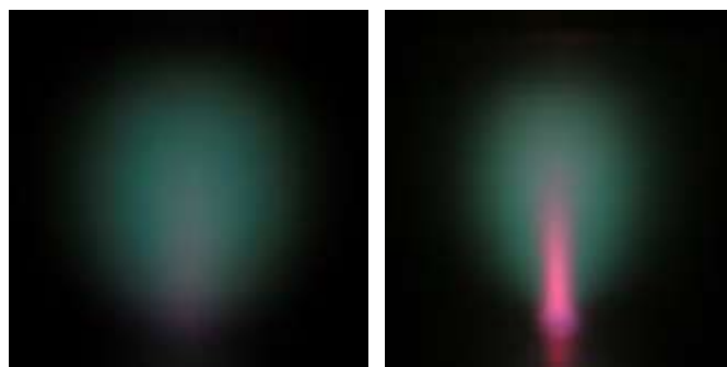
Figure 1. Contraction of microwave discharge with increasing pressure from 345 to 355 Torr.
